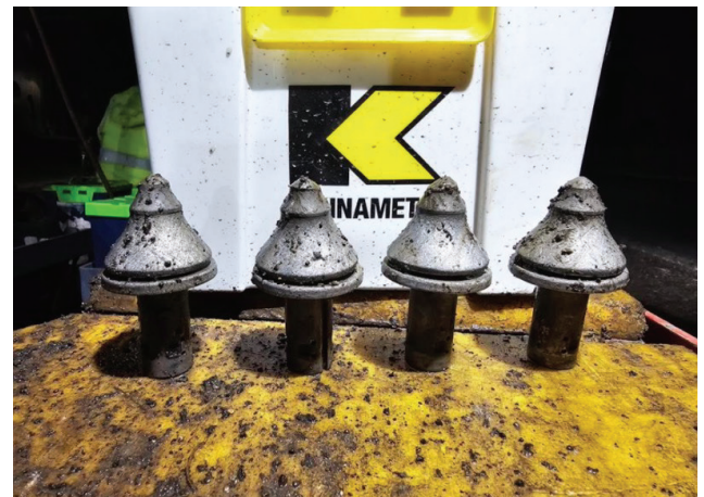
Kennametal RK52 picks at job completion. Body shape creates extra clearance under the tip and extra slope for holder protection.
